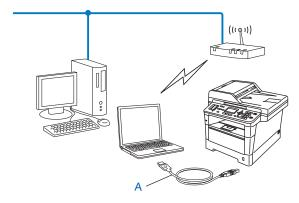
1 You can configure the wireless settings of the machine using a USB cable temporarily connected to a wired or wireless computer.
